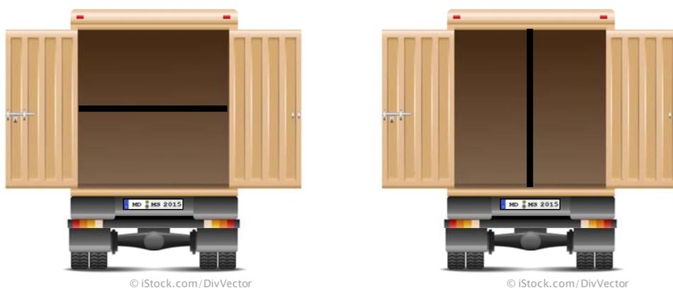
Figure 1: Double-deck loading and widthwise load compartments
